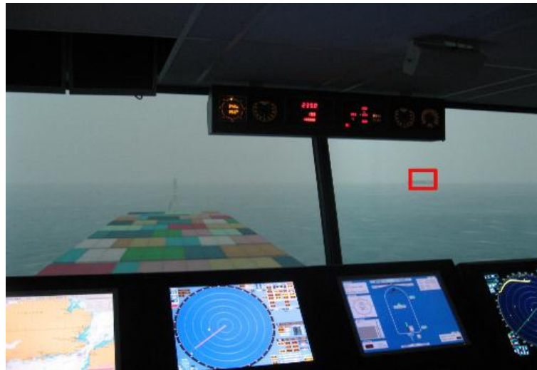
Figure 3 - Indication of dangerous target projected as a red box on the bridge window.
